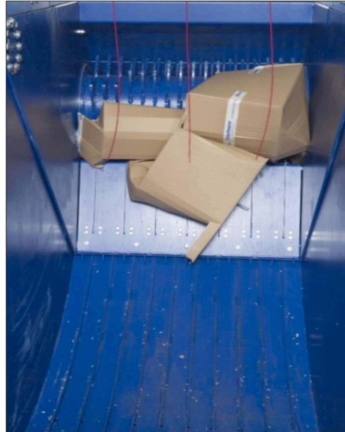
The turning rotor forwards the material into the press chamber.
