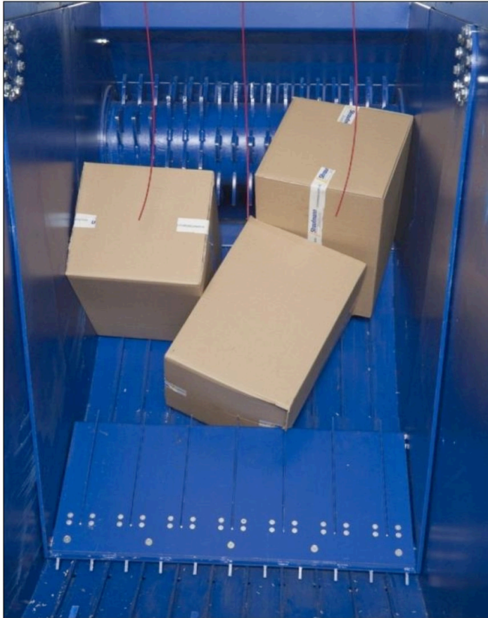
The swing moves back-/forwards and pushes the material to the rotor.
