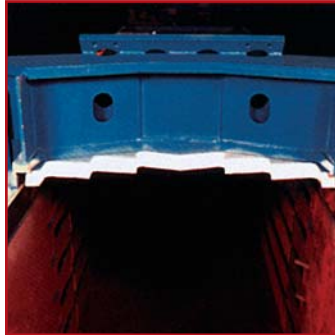
Robust 2-inch thick three-stage replaceable, shear blade eliminates the need for pre-processing.
