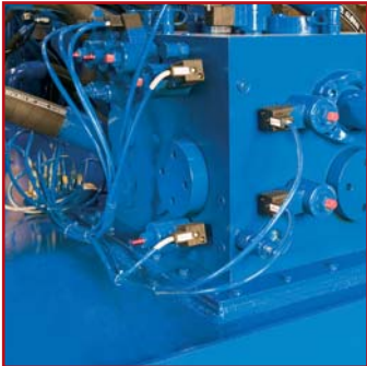
Ultramatic logic controlled manifold maximizes componentry yet simplifies the movement of oil throughout the baling cycle.
