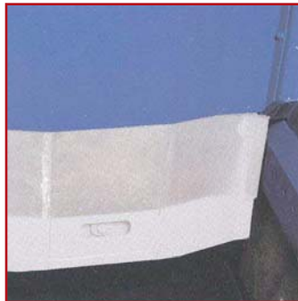
Stamper penetrates two-thirds of bale chamber for automatic shearing control.
