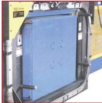
Ejector ram fully discharges finished bales for convenient forklift access.
