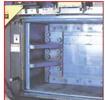
The Versa-Door provides over-size bale release, size control and bale separation.
