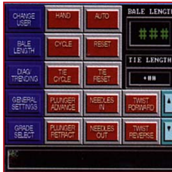
"Pathfinder" Touch Screen control panel uses graphics to guide operators through all baler functions.
