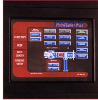
"Pathfinder" Plus Touch Screen operator interface simplifies baler controls and troubleshooting.
