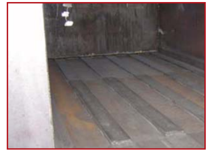
Hi-Low floor reduces material from getting under the platen.
